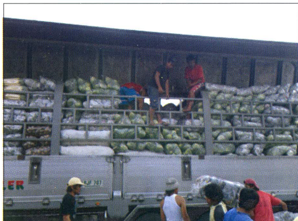
Figure 4: A truck design in the Philippines where the truck opens on both sides
